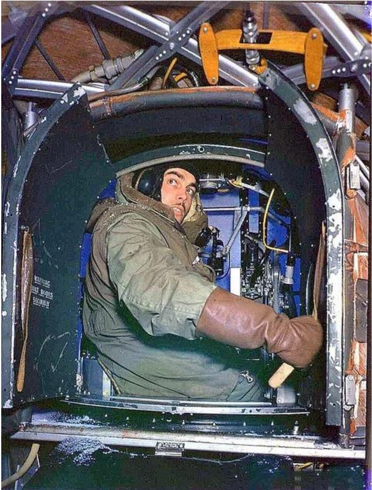
Frazier-Nash hydraulically powered front turret of the Vickers Wellington bomber, with it's two .303 caliber Browning machine guns.
