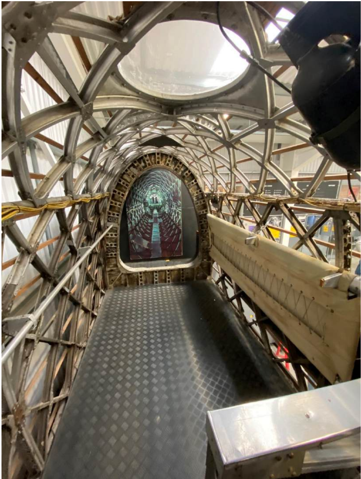
View towards the rear gunner's position, hammock for crew to rest and the navigators astro dome to take star fixes.
