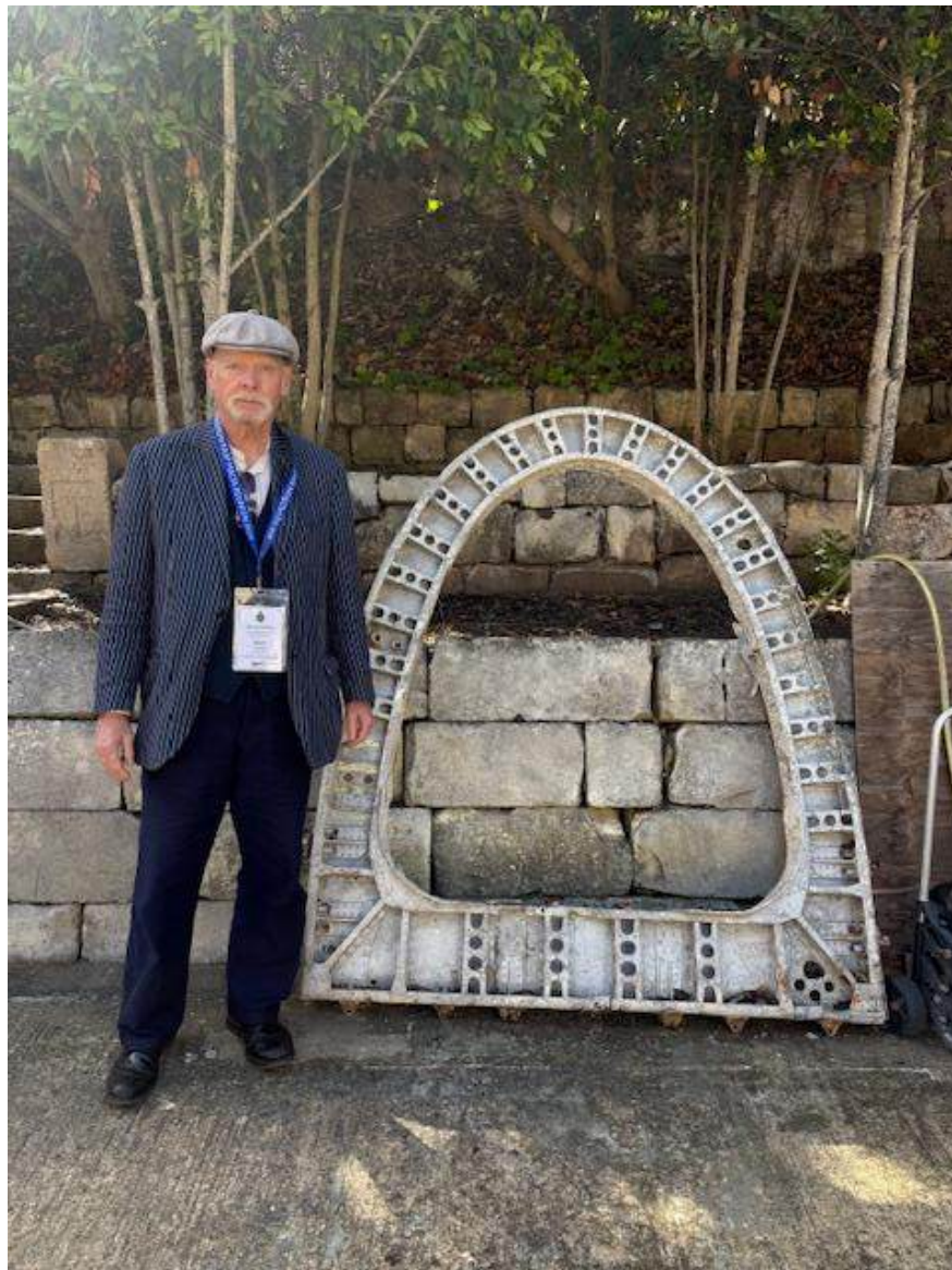
Adam Wagstaffe standing next to the Geodetic Wellington bulkhead, for reference. Pretty small space to crawl through. – at the Malta Aviation Museum.
