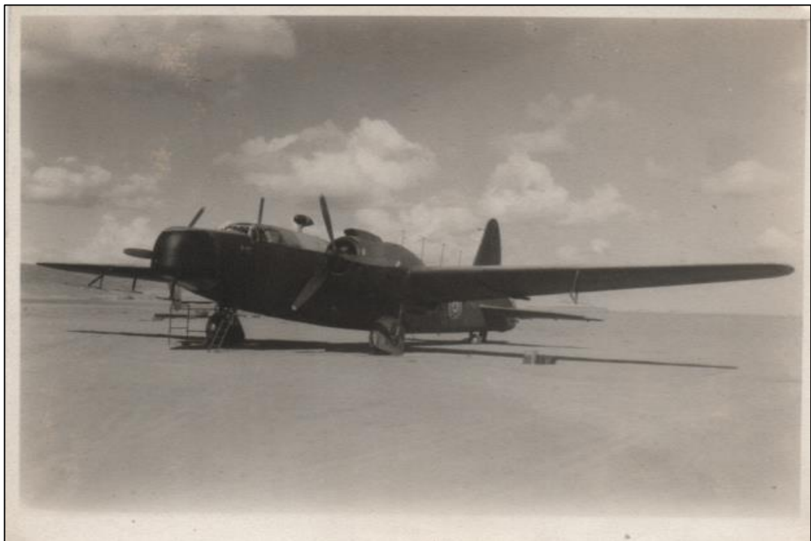
WELLINGTON MK XIII as torpedo bomber Tunisia 1943 (PROVILLE) (carrying 2 torpedoes)
